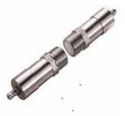
Microwave level detector provides a method of non-contact measurement, so it can be installed in silos, carrier pipes, rods or free fall extensions. According to different models, it can be applicable for a range of ( $0 \approx 8$ ) m with customized wider range. For any vessel shell or carrier pipe of non-metallic materials, measurement can be directly conducted from the outside.
